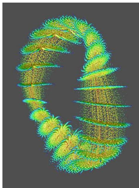
Fig. 3. The fast particle perpendicular pressure in a two-field period quasi-axisymmetric stellarator configuration in real space calculated from the corresponding moment of the hot helium-3 ion distribution function obtained with the VENUS code<sup>5</sup> for a case with high field side ICRH deposition.
