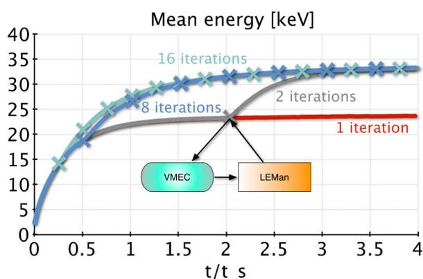
Fig. 2. The mean fast particle energy in JET after 1, 2, 8, and 16 iterations between the anisotropic VMEC/ANIMEC equilibrium, the ICRH wave absorption (LEMan), and the guiding center particle orbit minority ion distribution function (VENUS). The slowing-down time is denoted by  $t_{-s}$ .
