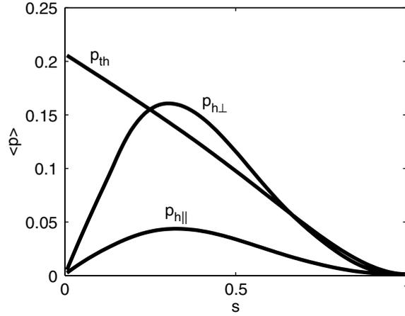
**Figure 1.** Typical flux surface averaged pressure profiles with HF side hot particle deposition and  $p_{\perp} > p_{\parallel}$ . The perpendicular (parallel) hot particle pressure is labelled as  $p_{h\perp}$  ( $p_{h\parallel}$ ) while the thermal pressure is  $p_{th} \equiv p(s)$ .
